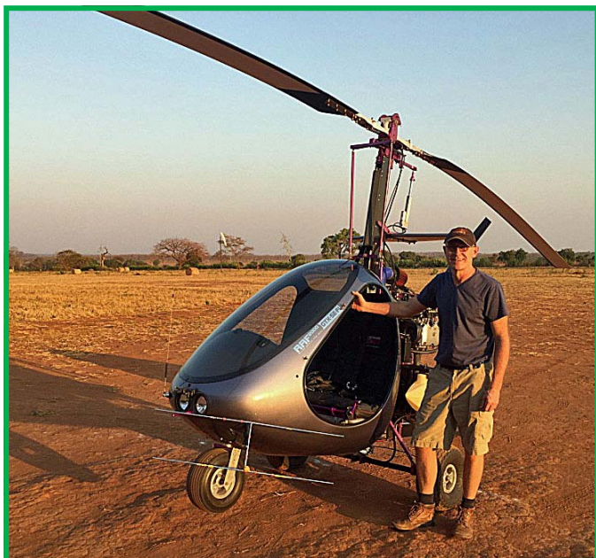
RAF 2000 gyrocopter, originally a Canadian design, now manufactured in South Africa. This ultra light aircraft features a non-driven rotary wing that aids in short take-off and landing. Note the two-element VHF antenna mounted on the nose to track radio-collared animals
